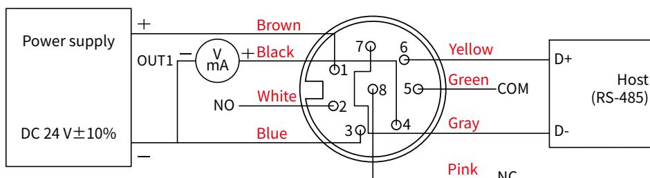
\*Please make sure the product and the device which connect with RS-485 are on common ground, avoid damaged product.
