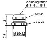
"increased safety" type cable gland for sensor mounting in partition barrier
