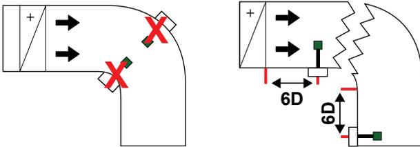
Place the sensor far enough away from bends, junctions or section changes in the duct to ensure an accurate reading.
