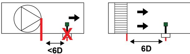
The preferred placement of the sensor is away from turbulent air caused by filters, rectifiers and coolers.
